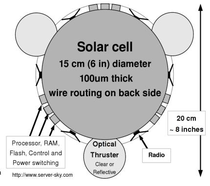
cost and makes a more effective solar sail. The current thickness target is 100 microns. Production silicon wafers are thinned to as little as 20 microns for some applications. 100 micron thick silicon is flexible, and can be rolled to diameters less than a centimeter without breaking. Future server-sats may become thinner than 10 microns, weighing less than a gram.
